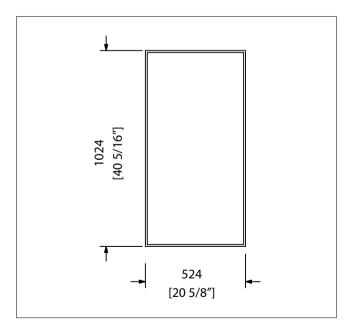
Mirror Heater is manufactured from a double insulated foil-element with a surface layer of polyester and a carbon-based heating element. One side is self adhesive for easy installation. Technical specifications: Rated voltage: 230V, Power 100W, Protection class: IP44, Connection cable: 2 m
