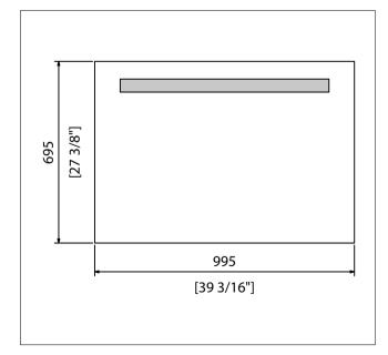
Mirror plain with light is manufactured from AISI 304 stainless steel and crystal. Mirror is 5mm thick crystal, silver plated, copper plated with varnish protection against corrosion, attached to base with special double-sided adhesive tape and silicon. Mirror mounts on wall with stainless steel screws. Mirror includes a T5 39W fluorescent lamp and electronic ballast 1x39W with 220V - 240V voltage.
