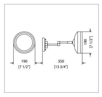
Wall mounted Magnifying Mirror with Light is manufactured from AISI 304 stainless steel and crystal. Magnifying mirror (x3) is 3mm crystal and attaches to frame. Support brackets use pivot hinges and attach to mounting base with stainless steel screws. Mounting flange attach to wall with stainless steel screws.
