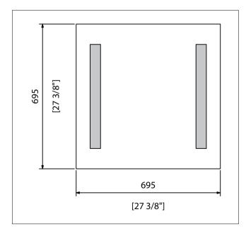
Mirror plain with light is manufactured from AISI 304 stainless steel and crystal. Mirror is 5mm thick crystal, silver plated, copper plated with varnish protection against corrosion, attached to base with special double-sided adhesive tape and silicon. Mirror mounts on wall with stainless steel screws. Mirror includes two T5 24W fluorescent lamp and electronic ballast 2x24W with 220V - 240V voltage.
