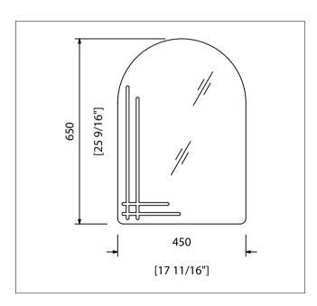
Naxos Mirror is manufactured from AISI 304 stainless steel and crystal. Mirror is 5mm thick crystal, silver plated, copper plated with varnish protection against corrosion, attached to stainless steel base with special double-sided adhesive tape and silicon. Mirror mounts on wall with stainless steel screws.
