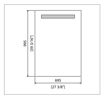
Mirror plain with light is manufactured from AISI 304 stainless steel and crystal. Mirror is 5mm thick crystal, silver plated, copper plated with varnish protection against corrosion, attached to base with special double-sided adhesive tape and silicon. Mirror mounts on wall with stainless steel screws. Mirror includes a T5 24W fluorescent lamp and electronic ballast 1x24W with 220V - 240V voltage.
