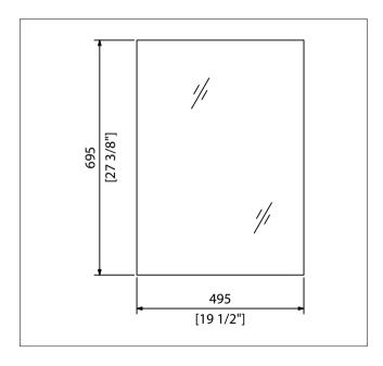
Plain Mirror is manufactured from AISI 304 stainless steel and crystal. Mirror is 5mm thick crystal, silver plated, copper plated with varnish protection against corrosion, attached to stainless steel base with special double-sided adhesive tape and silicon. Specially designed mounting system enables the mirror to be installed either vertically or horizontally without modification. Mirror mounts on wall with stainless steel screws.
