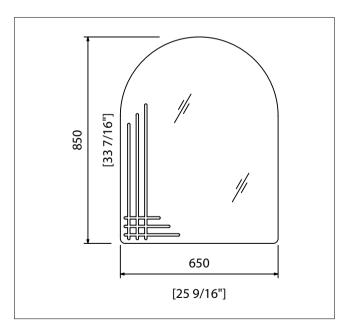
Santorini Mirror is manufactured from AISI 304 stainless steel and crystal. Mirror is 5mm thick crystal, silver plated, copper plated with varnish protection against corrosion, attached to stainless steel base with special double-sided adhesive tape and silicon. Mirror mounts on wall with stainless steel screws.
