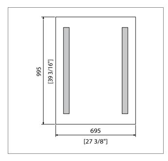
Mirror plain with light is manufactured from AISI 304 stainless steel and crystal. Mirror is 5mm thick crystal, silver plated, copper plated with varnish protection against corrosion, attached to base with special double-sided adhesive tape and silicon. Mirror mounts on wall with stainless steel screws. Mirror includes two T5 39W fluorescent lamp and electronic ballast 2x39W with 220V - 240V voltage.
