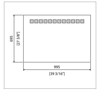
Mirror plain with light is manufactured from AISI 304 stainless steel and crystal. Mirror is 5mm thick crystal, silver plated, copper plated with varnish protection against corrosion, attached to base with special double-sided adhesive tape and silicon. Mirror mounts on wall with stainless steel screws. Mirror includes a T5 39W fluorescent lamp and electronic ballast 1x39W with 220V - 240V voltage.
