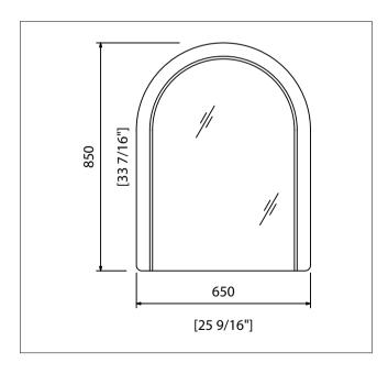
Sifnos Mirror is manufactured from AISI 304 stainless steel and crystal. Mirror is 5mm thick crystal, silver plated, copper plated with varnish protection against corrosion, attached to stainless steel base with special double-sided adhesive tape and silicon. Mirror mounts on wall with stainless steel screws.
