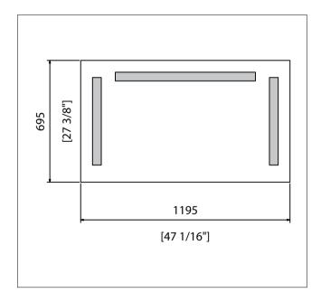
Mirror plain with light is manufactured from AISI 304 stainless steel and crystal. Mirror is 5mm thick crystal, silver plated, copper plated with varnish protection against corrosion, attached to base with special double-sided adhesive tape and silicon. Mirror mounts on wall with stainless steel screws. Mirror includes two T5 24W and one 39W fluorescent lamp and two electronic ballasts (one 2x24W and one 1x39W) with 220V - 240V voltage.
