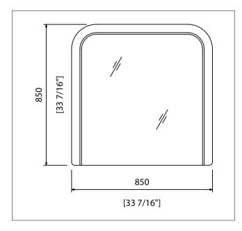
Tinos Mirror is manufactured from AISI 304 stainless steel and crystal. Mirror is 5mm thick crystal, silver plated, copper plated with varnish protection against corrosion, attached to stainless steel base with special double-sided adhesive tape and silicon. Mirror mounts on wall with stainless steel screws.
