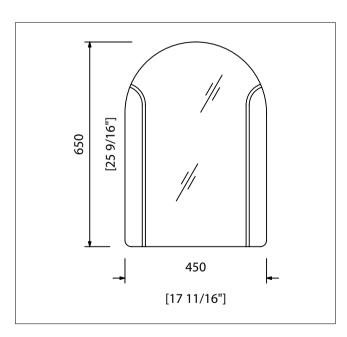
Paros Mirror is manufactured from AISI 304 stainless steel and crystal. Mirror is 5mm thick crystal, silver plated, copper plated with varnish protection against corrosion, attached to stainless steel base with special double-sided adhesive tape and silicon. Mirror mounts on wall with stainless steel screws.
