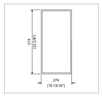
Mirror Heater is manufactured from a double insulated foil-element with a surface layer of polyester and a carbon-based heating element. One side is self adhesive for easy installation. Technical specifications: Rated voltage: 230V, Power 25W, Protection class: IP44, Connection cable: 2 m
