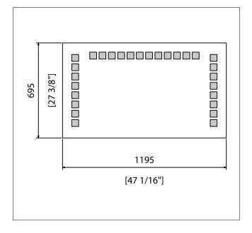
Mirror plain with light is manufactured from AISI 304 stainless steel and crystal. Mirror is 5mm thick crystal, silver plated, copper plated with varnish protection against corrosion, attached to base with special double-sided adhesive tape and silicon. Mirror mounts on wall with stainless steel screws. Mirror includes two T5 24W and one 39W fluorescent lamp and two electronic ballasts (one 2x24W and one 1x39W) with 220V - 240V voltage.
