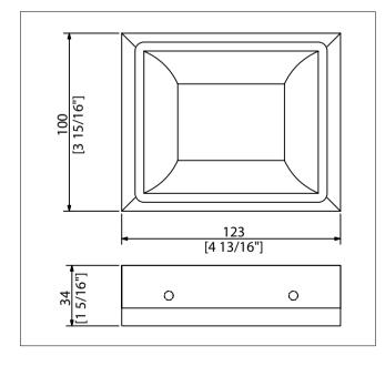
Wall mounted Ashtray is manufactured completely from AISI 304 stainless steel. Frame is 1.2mm thick and attaches to 1.2mm thick ashtray with stainless steel hinge. Frame securely attaches to wall with stainless steel screws. Ashtrays flips over for easy cleaning.
