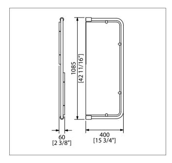
Urinal Separator is manufactured completely from AISI 304 stainless steel. Frame is 25mm tube, 1.5mm thick and is mechanically attached to solid stainless steel brackets. Panel is 2mm thick. Separator is securely attached to wall with four exposed stainless steel screws.
