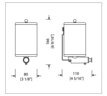
Liquid Soap Dispenser is manufactured from brass and AISI 304 stainless steel. Container is 1.5mm thick brass. Pump is solid brass and operates with stainless steel spring. Dispenser is mounted to wall with 1.2mm thick mounting flange and stainless steel screws.
