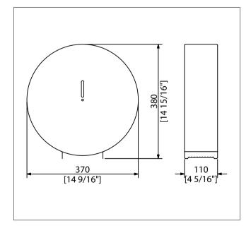
Jumbo Roll Paper Dispenser is completely manufactured from 0.8mm thick AISI 304 stainless steel. It securely attaches to wall with two stainless steel screws.
