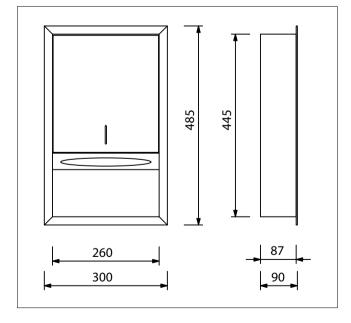
Recessed Paper Towel Dispenser is manufactured completely from 0.8mm thick AISI 304 stainless steel. Paper Towel Dispenser has a capacity of 300 C-fold paper towels. The cover attaches to cabinet with stainless steel pivot and locks with concealed stainless steel lock. The cover has a slot that indicates refill time. The required wall opening for recession is 265 mm x 455 mm with a depth of 90 mm.
