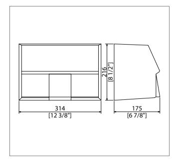
Hand Dryer with Photocell is manufactured from 1.2mm thick AISI 304 Stainless Steel. Operation is automatic due to an electronic sensor. Electrical Characteristics: Voltage: 220/240V Heating Element: 2100W Overall power absorption: 2200W Air flow: 4.6 m3/min Noise Level: 61-67 dBA
