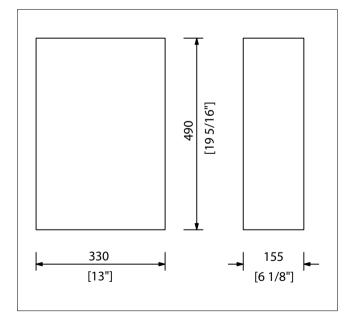
Waste Receptacle is completely manufactured from 0.8 mm thick AISI 304 stainless steel. Capacity is 25lt. It securely attaches to wall with two stainless steel screws.
