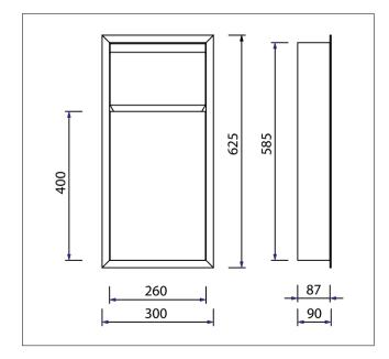
Recessed Waste Receptacle with lid is manufactured completely from 0.8mm thick AISI 304 stainless steel. The Waste Receptacle is removable for easy cleaning. The lid attaches to cabinet with stainless steel pivot. The required wall opening for recession is 265 mm x 605 mm with a depth of 90 mm.
