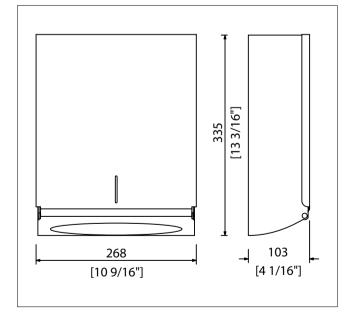
Paper Towel Dispenser is completely manufactured from 0.8mm thick AISI 304 stainless steel. Cover attaches to cabinet with stainless steel pivot and locks with concealed stainless steel lock. Cover has slot that indicates refill time. The capacity of the dispenser is 300 C-fold paper towels. It securely attaches to wall with three stainless steel screws.
