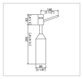
Liquid soap dispenser for table top mounting, into worktops with max. 45 mm thickness, high polished chromated brass, requires 22 mm drilling hole, 1/2 thread, spout not movable, spout length 140 mm, suitable for liquid soaps and lotions, 1 litre soap tank with membrane for pressure balance, filled from above.
