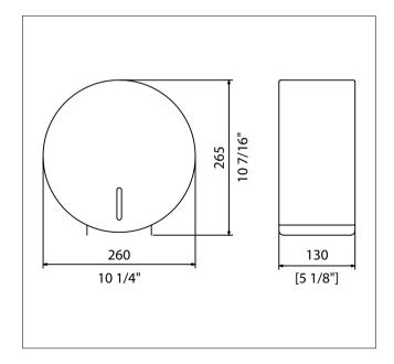
Jumbo Roll Paper Dispenser is completely manufactured from 0.8mm thick AISI 304 stainless steel. It securely attaches to wall with two stainless steel screws.
