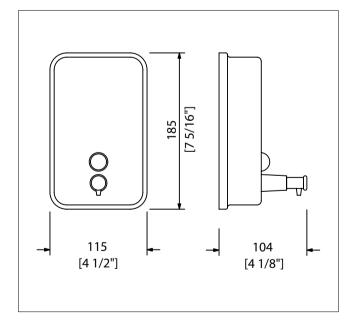
Liquid Soap Dispenser is manufactured from AISI 304 stainless steel. Container is 0.8mm thick and is equipped with a transparent refill indicator. The internal mechanism of the pump is manufactured from high quality platic and operates with stainless steel spring. Dispenser is mounted to wall with 1.2mm thick mounting flange and stainless steel screws.
