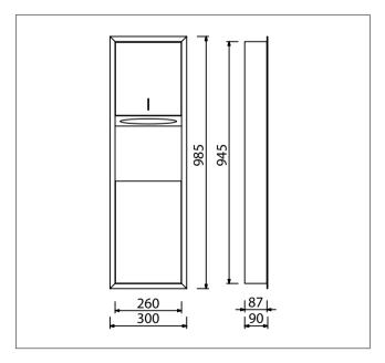
Recessed Paper Towel Dispenser and Waste Receptacle combination is manufactured completely from 0.8mm thick AISI 304 stainless steel. Paper Towel Dispenser has a capacity of 300 C-fold paper towels. The cover attaches to cabinet with stainless steel pivot and locks with concealed stainless steel lock. The cover has a slot that indicates refill time. The Waste Receptacle is removable for easy cleaning. The required wall opening for recession is 265 mm x 955 mm with a depth of 90 mm.
