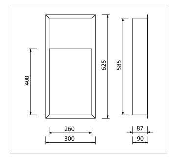
Recessed Waste Receptacle is manufactured completely from 0.8mm thick AISI 304 stainless steel. The Waste Receptacle is removable for easy cleaning. The required wall opening for recession is 265 mm x 605 mm with a depth of 90 mm.
